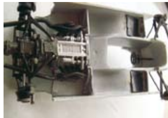
Underside. Note plastic card bracing & Tamiya radiators
