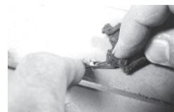
17 Support delicate white-metal pieces by laying them on a piece of thick glass while carefully polishing them with steel wool.
