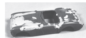
11A There may be a number of surface blemishes visible after the first primer coat; fill the larger ones with 2-part putty.
