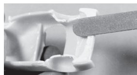
3 Common emery boards make great "files" for cleaning up resin kits. Use sandpaper to smooth the "filed" surfaces.
