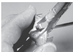
5A Half-round files work best for removing mould lines from the inside of body shells.
