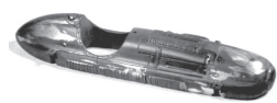
14 The body of this Novi had many small "blemishes", none large enough to require filler. Simply sanding the general area to bare metal and spraying on another coat of primer produced a smooth surface. Some models may need to have this repeated a couple of times.
