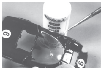
24 Apply adhesive for vac-forms with a small, thin paintbrush. If necessary, glue one side in place and let it dry overnight before gluing the second side.
