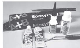
2 Both white-metal and resin kits require either epoxy or "super glue" to bond the parts together - plastic cement will not work.
