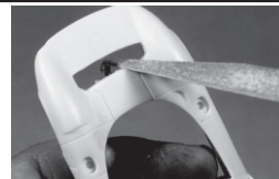
8 Emery boards can be cut with scissors to create the shape you need to get into small openings in castings.
