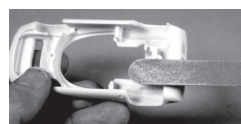
7 Common emery boards make great "files" for cleaning up resin kits. Use sandpaper to smooth the "filed" surfaces.
