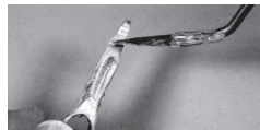
4 Glue as much of the body together as possible - remember - engines, interiors, etc. must be fitted later - & fill the seams with putty.
