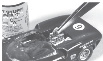
28 Good tweezers are a "must have" tool for building 1/43 scale models; all too often the spot where a piece must go is too small for fingers.
