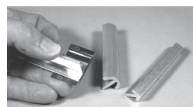
20 A variety of hard smooth surface shapes are very useful for bending photo-etched pieces.
